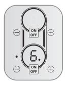
③ If the Cooking Zone or pads are held for more 10 seconds, the timer display will show the error message . To clear this error message, press the ON/OFF pad for the Cooking Zone you were setting. This message does NOT relate to the timer pad.
